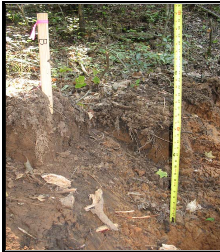
PHOTO 9: Exc. Depth Measurement – Stake B = 1.33 ft DATE: 8/7/09 VIEW: North
