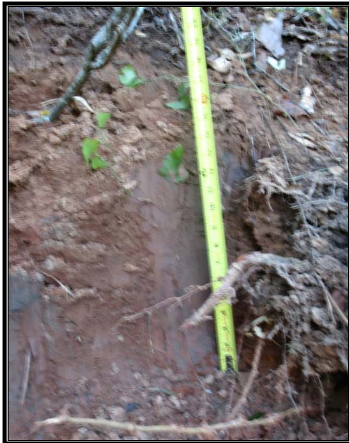
PHOTO 17: Exc. Depth Measurement – Stake F = 1.25 ft (Notes: Stake Not Shown.)
