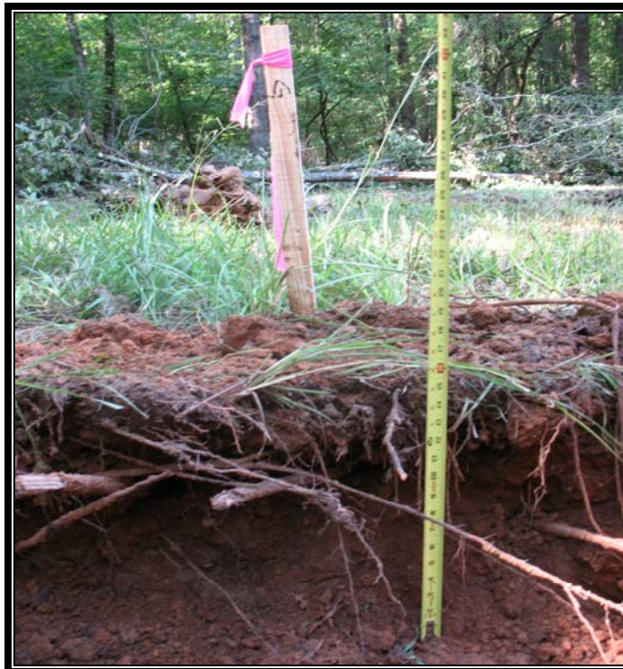
PHOTO 18: Exc. Depth Measurement – Stake G = 1.33 ft
