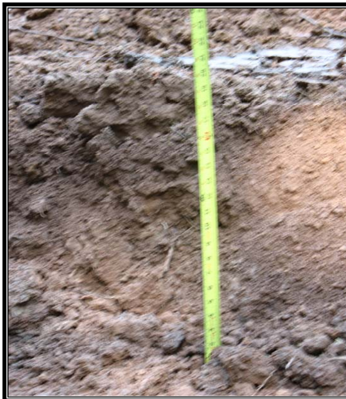
PHOTO 20: Exc. Depth Measurement – Stake I = 1.33 ft (Notes: Stake Not Shown.) DATE: 8/7/09 VIEW: West
